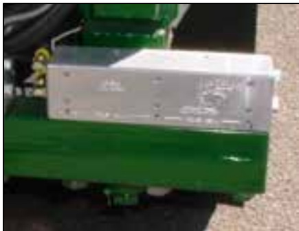
Tri-cylinder Poppet Valves have no external moving parts
